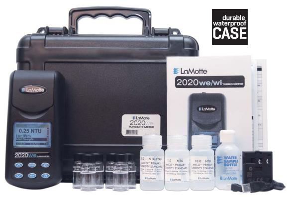
Kits are supplied with 0, 1, and 10 NTU standards, sample bottle, six sample tubes, USB cable and wall adapter.
